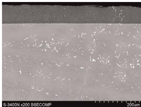
Figure 57. General cross-section view on the sample MAR 247 LC with AlSi coating before testing.
