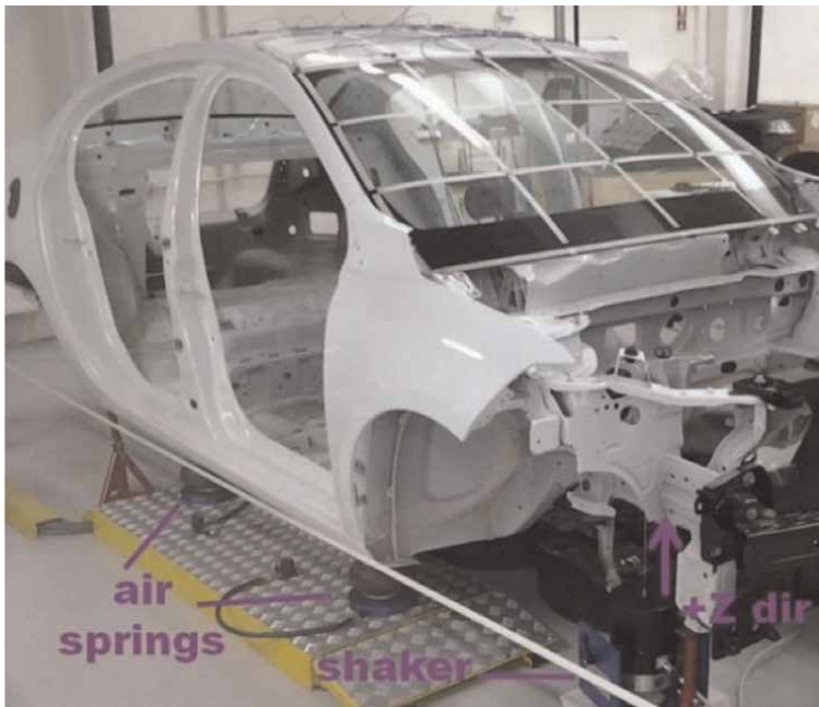
Figure 13. Full vehicle modal test set-up [17].
