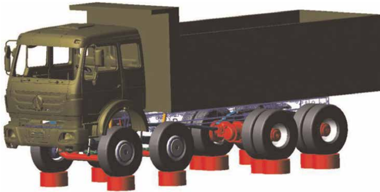
Figure 11. Multi body truck model [15].
