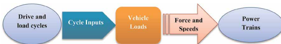
Figure 1. Information flow in a kinematic or backward HEV model [11].
