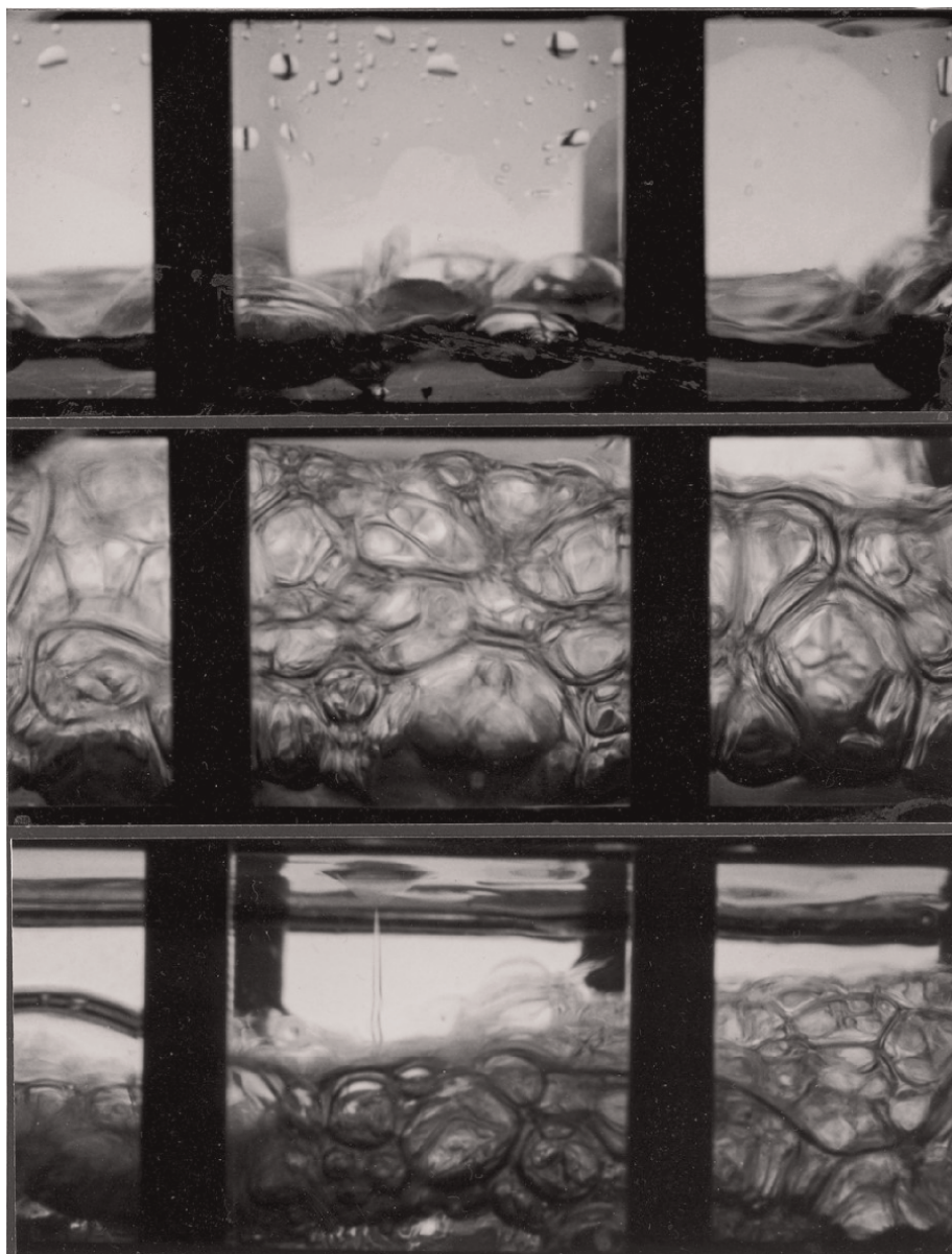
Figure 3. Nucleate pool boiling of water on horizontal copper plate (see Figure 5 for test section and electron-microscope images of boiling surfaces use in this experimental setup) at sub-atmospheric pressures: Parameters of working fluid—volume 120 ml and level 5.8 mm; height of boiling-condensation chamber 38 mm; scale—pitch between two thread-rods (black vertical posts on photos) equals to 40 mm.
