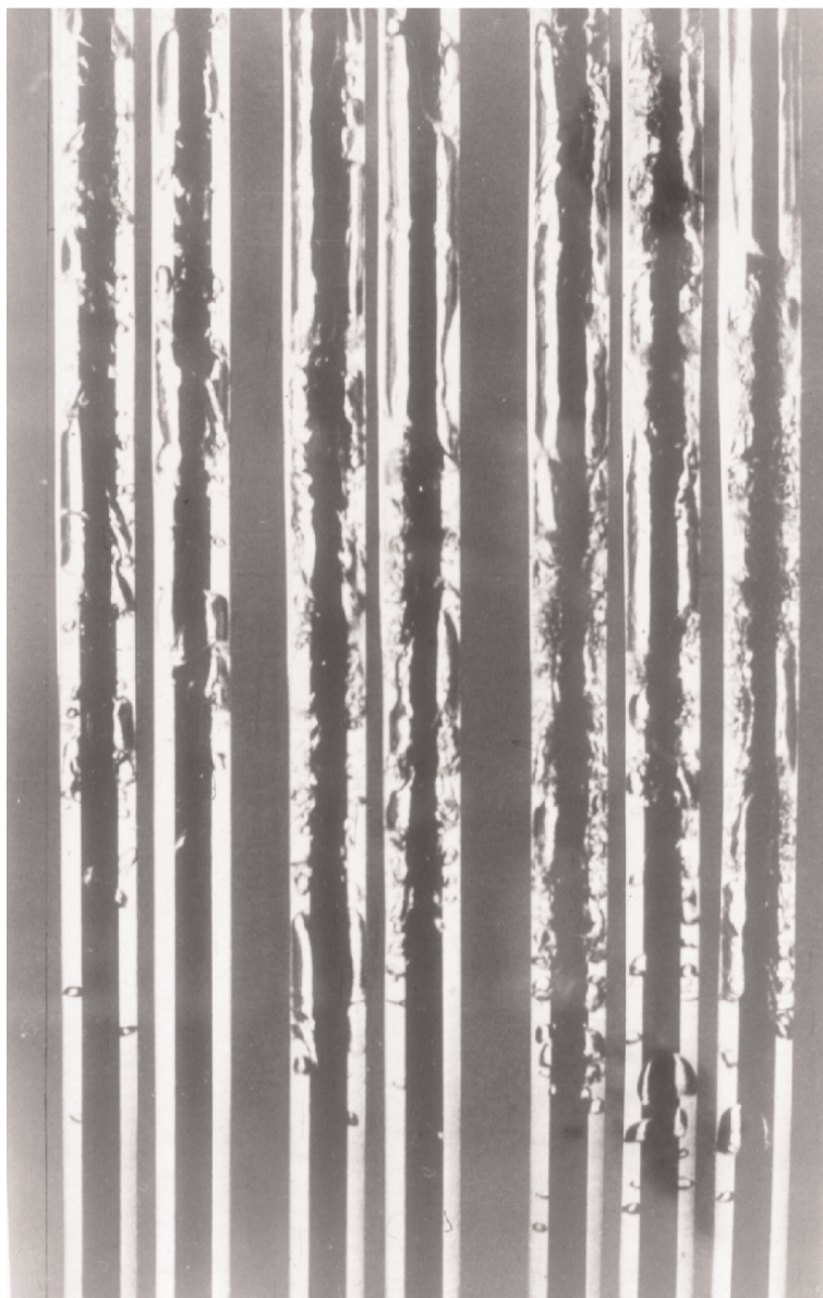
Figure 11. Nucleate boiling in two-phase counter-flow thermosyphon on metal heated rod (annular-channel evaporator): Water, atmospheric pressure, filling charge 100% of evaporator volume, and heat flux increasing from left to right up to critical heat flux (CHF).
