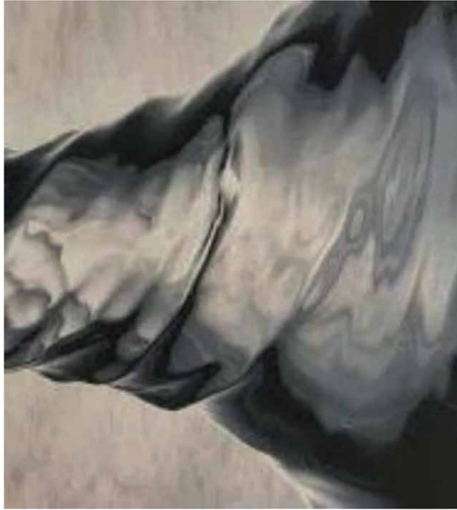
Figure 3. Corkscrew flow configuration. View of a corkscrew vortex flow in fluid dynamics. Its geometry is equivalent to that expected for a vortex flow in the Venus wake with its width and position varying during the solar cycle. The vortex flow becomes thinner along the radial direction in the wake axis when measured on a plane transverse to that of the figure further downstream from Venus [5].
