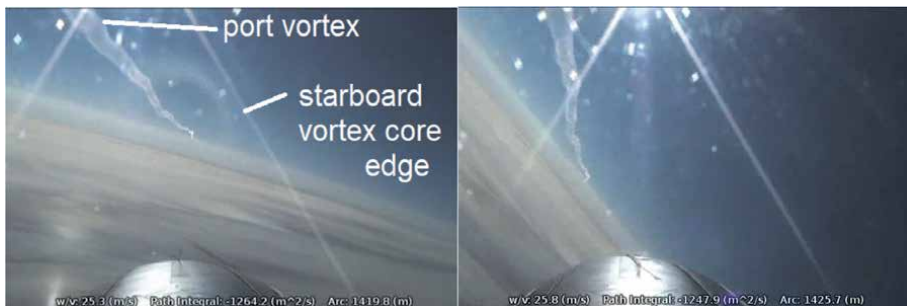
Figure 4. vortex core entry (left) and exit (right) of the curved-inwards, near-vertical traverse through the starboard vortex core of an A388 aircraft, of duration 0.7 sec. Overlaid data indicated core edge vortex velocity was 26 m/s, circulation as per Figure 3 , crossplane flight path distance was 6 m; circular reconstruction of the core identified a core radius of 3.6 m [9].
