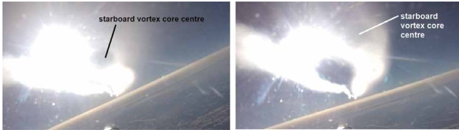
Figure 25. Into-sun view of trailing vortices from an A388 jet transport, centred directly below the starboard vortex core.
