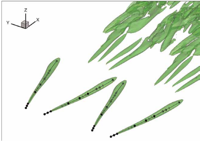
Figure 15. Selected seed points and corresponding forward Liutex gradient lines.
