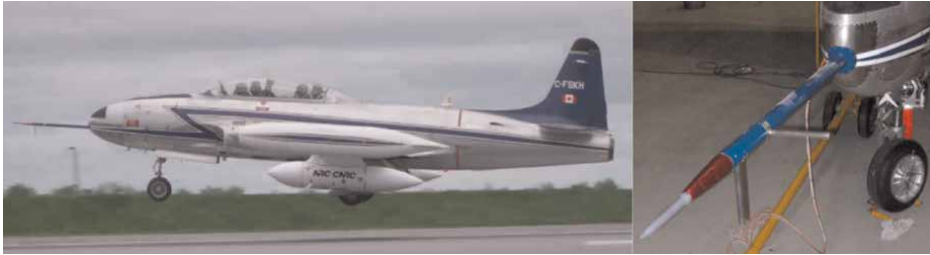
Figure 1. NRC. CT-133 research aircraft; close-up view of air data nose-boom, including pitot-static tube, and cylinders in cross-flow for flow angle measurement.
