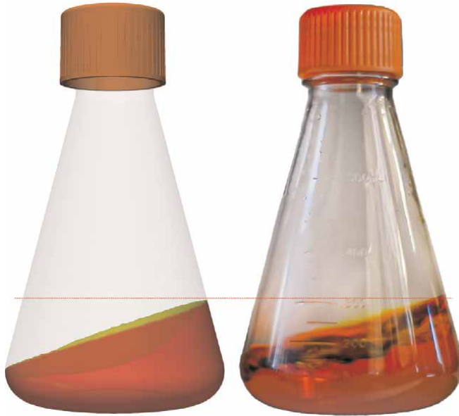
Figure 9. Simulation (left) and experiment (right) of the fluid flow in a 500 mL shake flask with 150 mL of working volume at 160 rpm and 25 mm shaking amplitude. The dashed red line indicates the empirically calculated maximum fluid height according to Büchs et al. [33], which deviates by only 2% from the simulated one.
