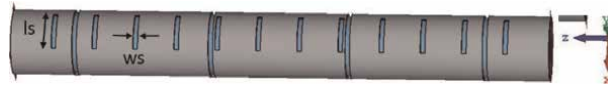
Figure 27. Slotted waveguide geometry, small slot for 4 GHz antenna ( l_s = 40 mm, w_s = 5 mm) and large slot for 1 GHz antenna ( l_s = 150 mm, w_s = 5 mm).
