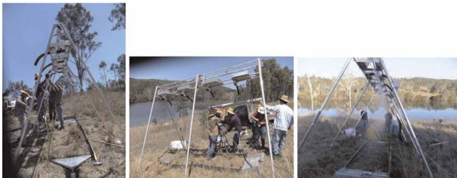
Figure 3. The Griffith University portable rainfall simulator (port-RFS) installation and operation in the field.
