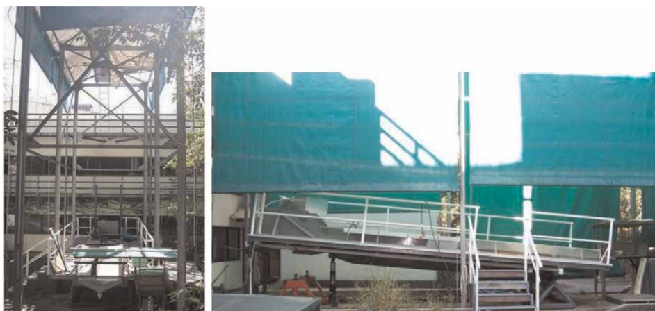
Figure 2. The Griffith University tilting flume simulated rainfall (GUTSR). The left picture shows the rainfall generator above the flume. The right picture shows a side view of the sloping flume and the wind shield.
