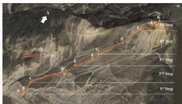
Figure 13. Five-steps appeared in the Tsaoling shear failure planes during the Jiji earthquake [11, 12].
