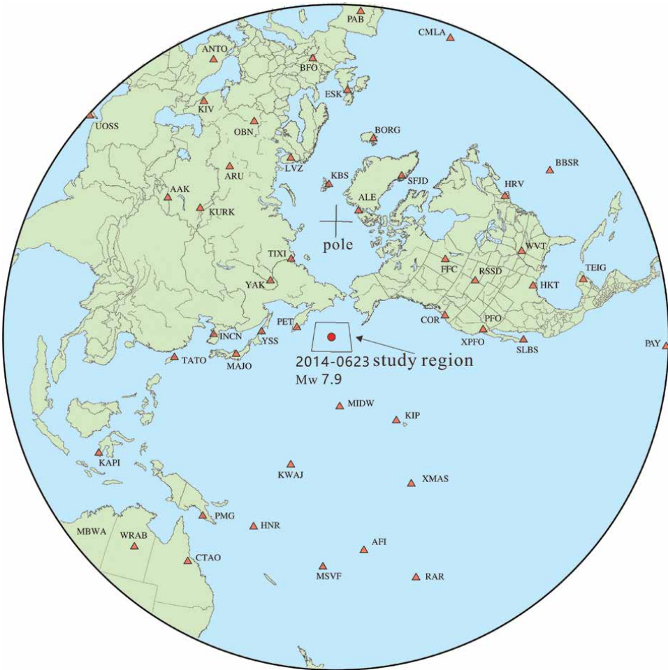
Figure 1. The location of the 23 June 2014 M_W 7.9 earthquake and the study region in the global setting. The red solid circle at the center shows the epicenter. The trapezoid shows the study region. The triangles show the positions of the seismic stations, at which the recorded mantle Rayleigh-wave seismograms were selected for the moment tensor inversion. The cross sign shows the location of the north pole.
