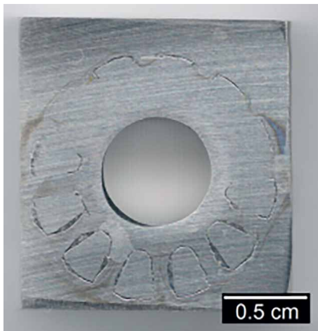
Figure 4. The crevice corrosion in metals [10].
