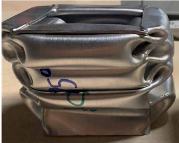
(b) Standing wave cooling after extrusion. OK condition and small crack formation on folds. (OK criteria is defined according to the OEM Company specs)
