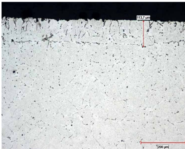
Figure 9. Typical ISZ formation on the 6063 aluminum alloys. (Image copyright © belongs to TRI METALURJI A.S.).
