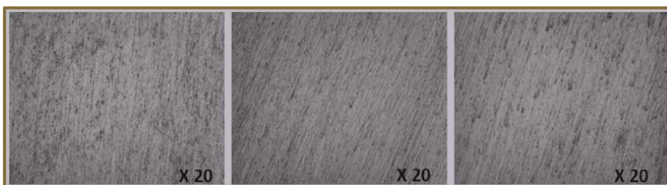
Figure 17. Micrographs of the friction stir layer taken twice at a cutting depth of 100 \mu\text{m} and at 80 mm/min in linear motion and 800 rpm in rotation.
