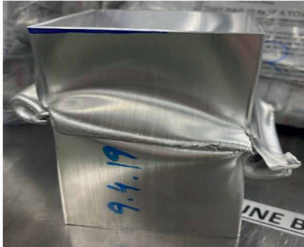
(a) Air cooling after extrusion. NOK condition due the crack formation on folds.
