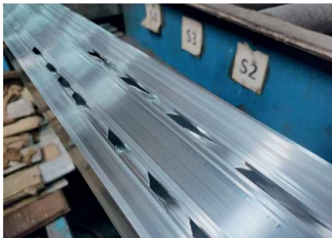
Figure 4. Bubble or blister appearing on extrudate surface.
