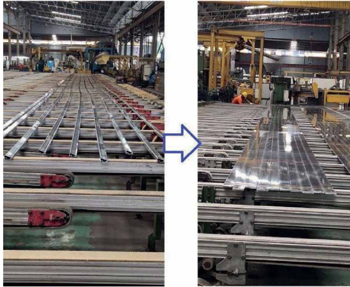
Figure 16. Good vs. bad materials stacking on conveyor table.
