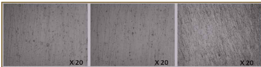
Figure 10. Micrographs of the friction stir layer cut once at a depth of 50 µm at an 800 rpm rotational speed and an 80 mm/min linear speed.
