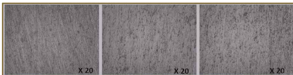
Figure 16. Micrographs of the friction stir layer taken twice at a cutting depth of 50 \mu\text{m} and at 80 mm/min in linear motion and 800 rpm in rotation.
