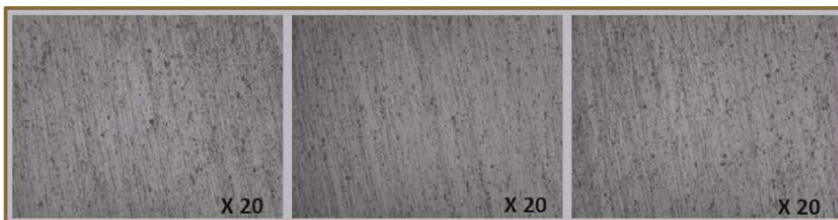
Figure 15. Micrographs of the friction stir layer taken twice at a cutting depth of 25 \mu\text{m} and at 80 mm/min in linear motion and 800 rpm in rotation.
