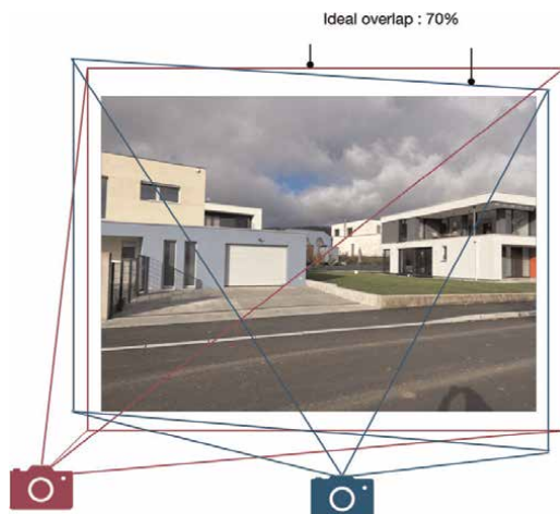
Figure 4. Ideal overlap to respect when capturing built environment.
