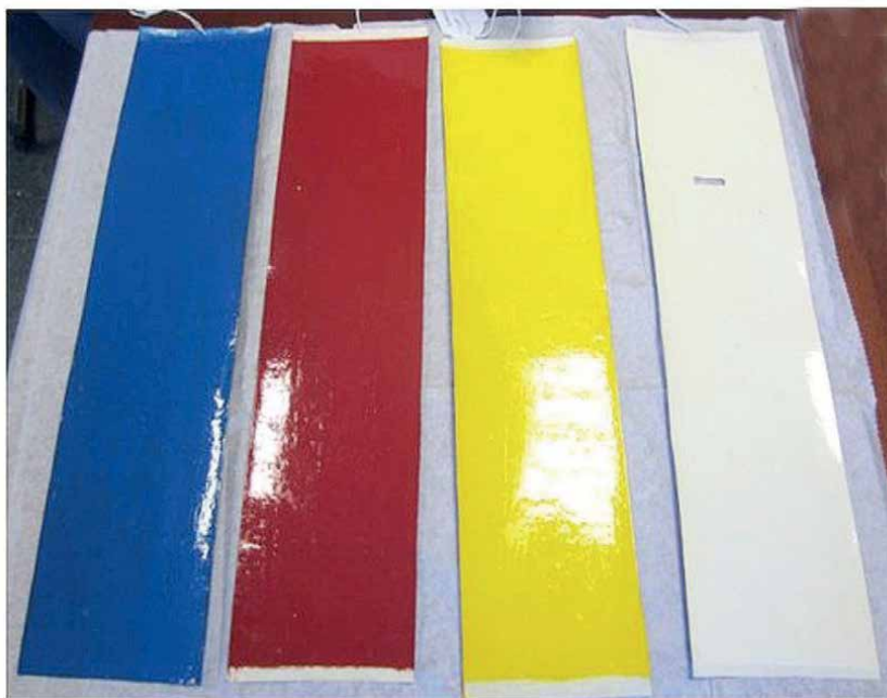
Figure 2. Reference samples: cobalt blue, cadmium red, cadmium yellow and lead White varnished with mastic.
