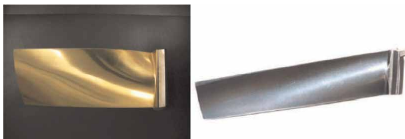
Figure 8. I & II generation coating (TiN series) III generation coating (TiAlN series) [44].
