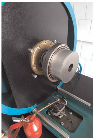
Figure 11. Appearance of the installed bearing for vibration measurements by the built-in sensors of the bench.
