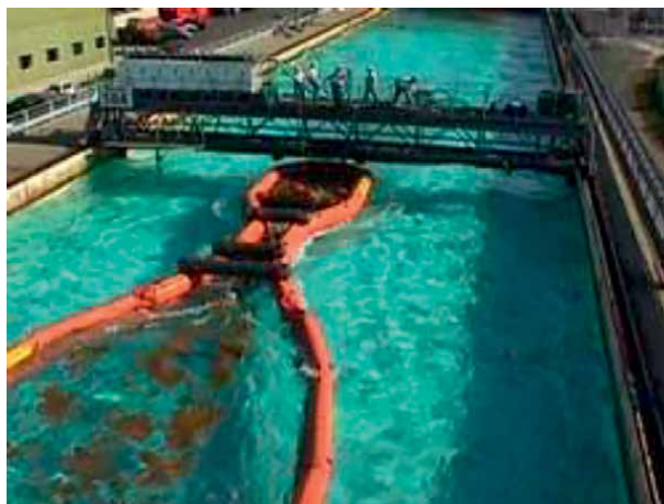
Figure 4. The oil containment boom in a ship lock [14].
