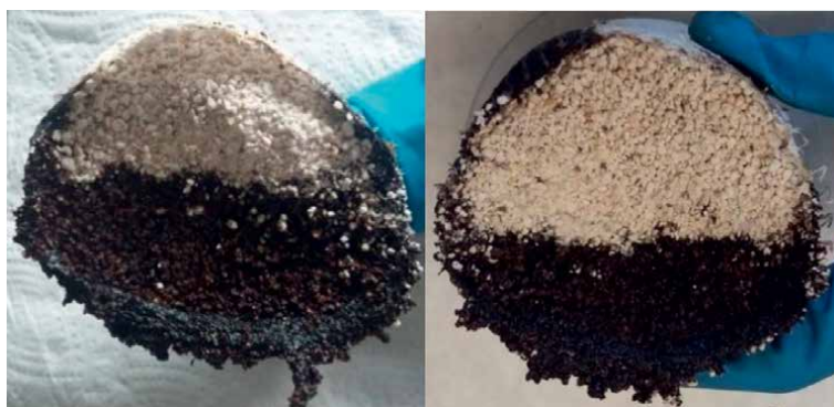
Figure 9. The absorption sock after absorption of crude oil (left) and oil from the water/oil mixture(right).
