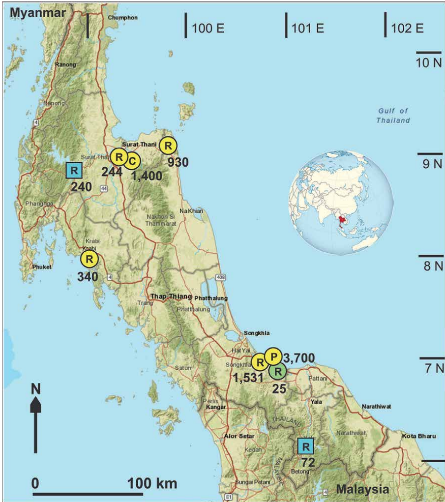
Figure 2. Electricity generation in Southern Thailand. Status: R = running, operating; C = under construction; P = planned. Fuel source: Yellow = oil, gas; green = biomass; blue-hydro. Power: Values next to symbols, in MW (further information and references in the text). Globe via [7].
