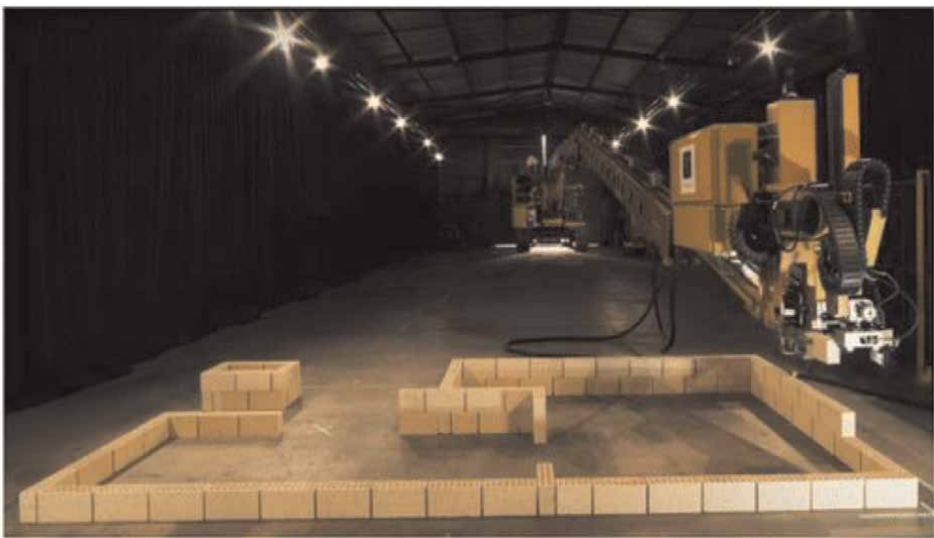
Figure 5. Bricklaying robot “HADRIAN X.” source: Pivac and Pivac [44].
