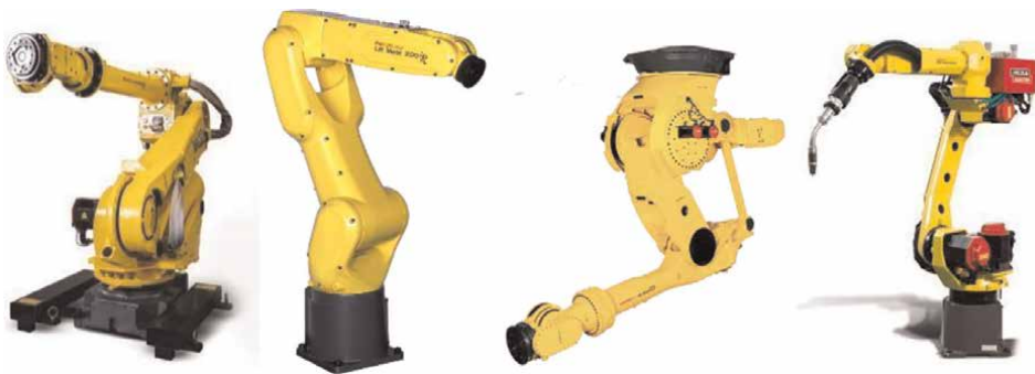
Figure 8. The FANUC M-10ia and the FANUC R-2000ib six-axis robots.
