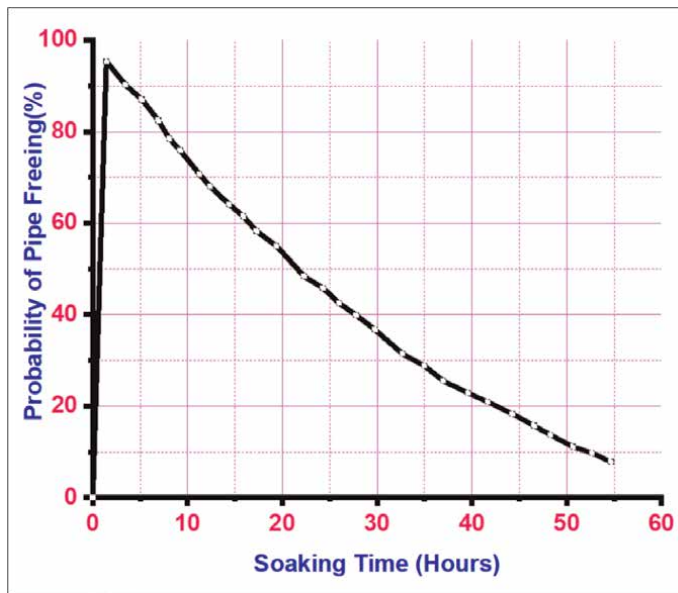
Figure 11. The probability of freeing the pipe against soaking time.
