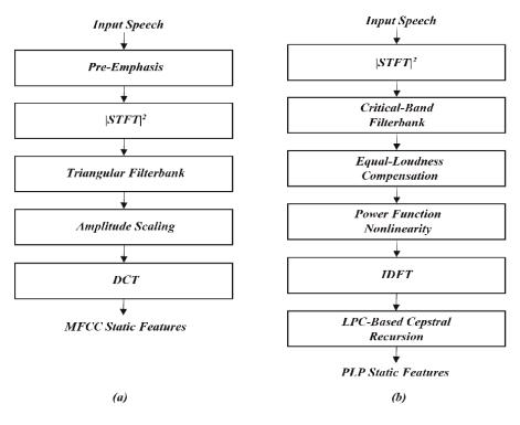
**Figure 1.** *Comparison of the MFCC (a) and PLP (b) structure.*
