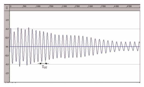
**Figure 8.** *A sound "A" at the 50th level of decomposition (frequency range is 51–250 Hz).*
