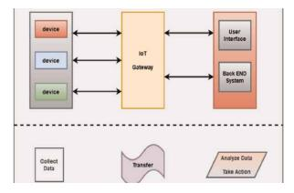
**Figure 1.** *IoT reference architecture [8].*
