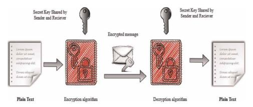
Figure 9. Simple symmetric model [9].
