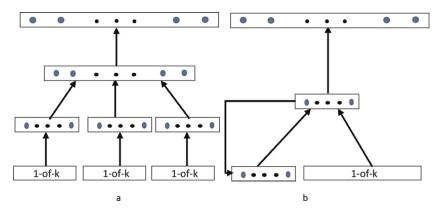
**Figure 1** *FNN vs. RNN architecture, a) FFNN and b) RNN.*
