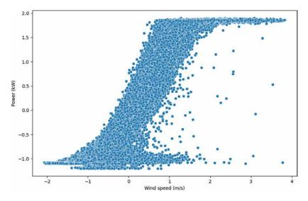
Figure 1. Power curve, relating the wind speed and the power generated by the turbine.
