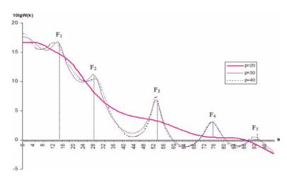
Figure 12. The Logarithmic power spectrum of LPC of a sound "A" at different orders of prediction p.
