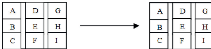
Figure 4. Non-duplicate mode: remains same as original image (no additional row and column).
