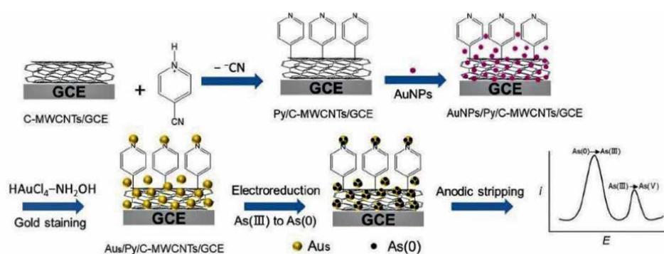
Figure 6. Preparation of the electrode [28].
