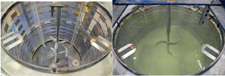
Figure 4. Photographs of a 1-m diameter tank equipped with ERT electrodes. Two different impeller configurations shown: Baffled and unbaffled.
