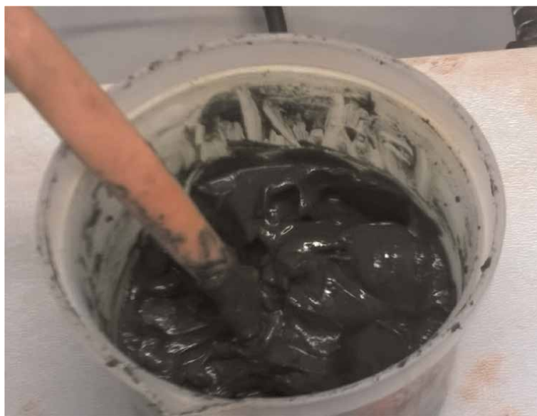
Figure 6. Viscous leach conditions from batch test.
