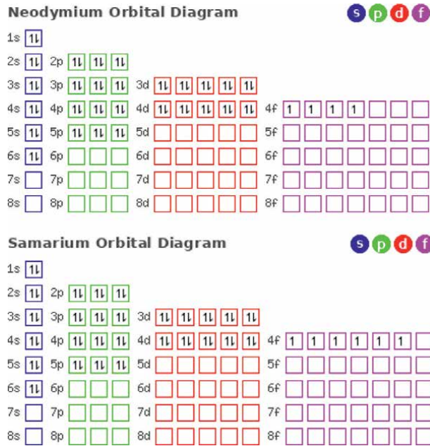
Figure 4. Electron configuration on orbital diagrams for rare earth elements neodymium and samarium [16].
