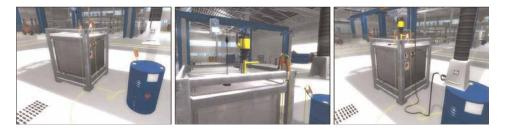
Figure 10. A pump is installed, grounding cables are attached, and a pipe leads to the barrel.
