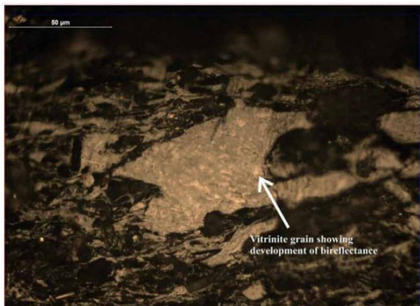
Figure 10. Photomicrograph of a heat-affected lower Permian Barakar formation shale from Raniganj basin, India, showing the development of bireflectance in vitrinite [33].
