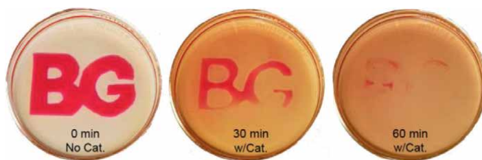
Figure 5. Depolymerization of Wacker Elastosil to cyclic siloxanes in a tetrabutylammonium fluoride THF bath [63].
