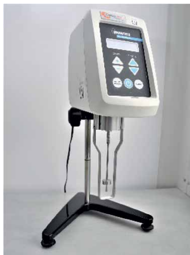
Figure 7. Brookfield viscometer with spindle number 62. Apparatus in that configuration and rotation speed of 60 rpm has measuring range 50 – 500 cP.
