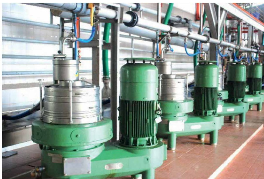
Figure 2. Centrifuges used in processing of natural rubber latex.
