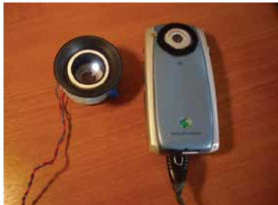
Fig. 6. An 'Eye Cup' with a Luminous Diode links to the Sony Ericsson P800 Mobile Phone
