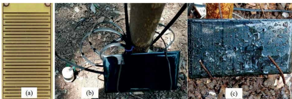
Figure 4. Sprayed water (a) to a wetness sensor, (b) to a dry solar cell, and (c) to forming drops in solar cell.
