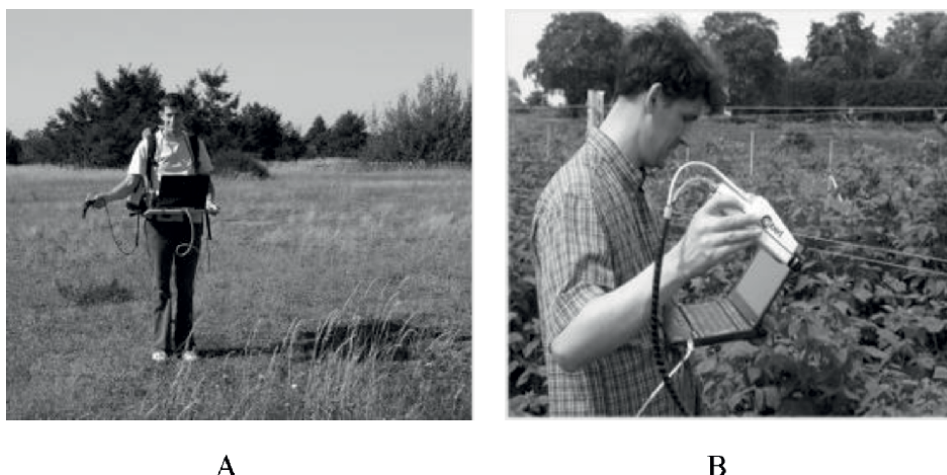
Figure 1. A non-imaging (A) and an imaging spectrometer (B) in field use. Source: A. Jung.
