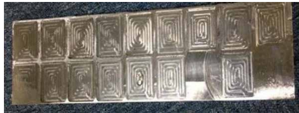
Figure 8. Machining profile on aluminium alloy 7075 material.
