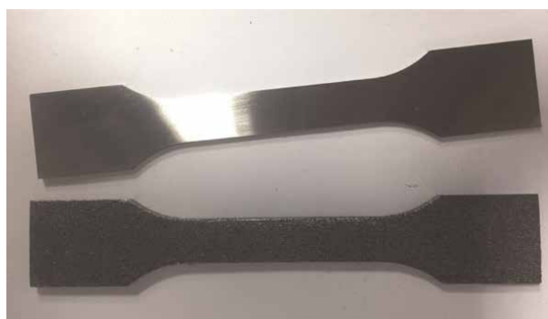
Figure 6. Sample with roughness removed (top) and untreated (bottom).
