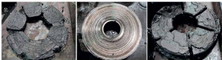
Figure 16. Examples of protector thrust bearing/runner damages.
