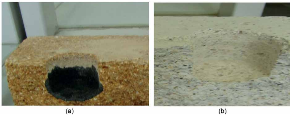
Figure 4. The results of the corrosion resistance cup test of refractory material to molten aluminum (Mg alloy). a – Conventional refractory fireclay shamoto brick; b – Special refractory with anti-wetting (for molten aluminum) additives (almost undamaged).
