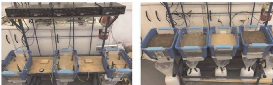
Figure 2. (a) electroosmotic drainage cell; and (b) gravitational drainage cell [35].
