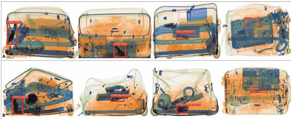
Figure 5. Exemplar detection of prohibited items in red box using Faster R-CNN [8] and trained on (A) Dbfg3 Real and (B) Dbf3 SC images.
