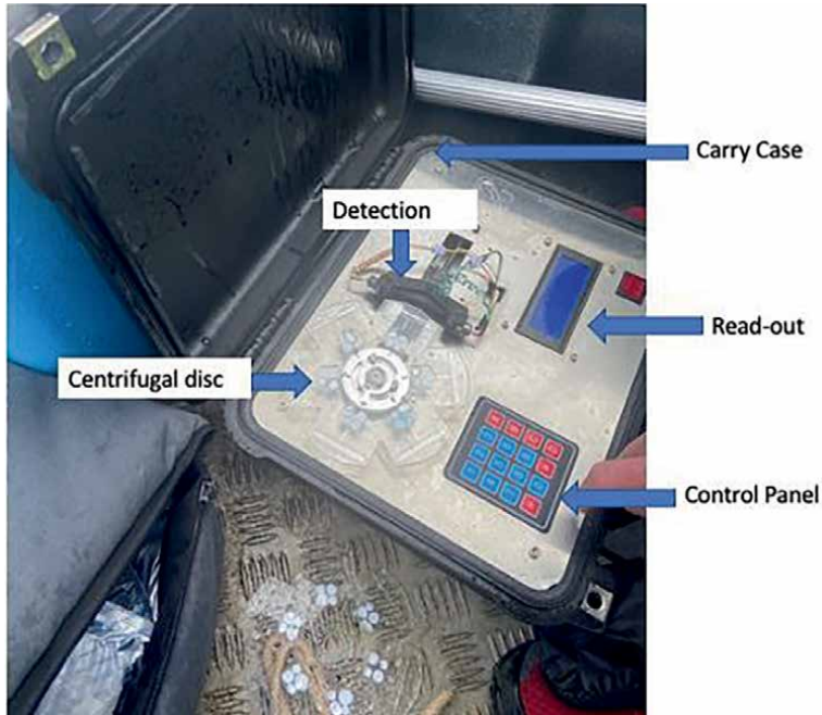
Figure 3. Image showing the use of the phosphate analyser onboard a boat—showing the keypad below the centrifugal platform and the read-out to the right.
