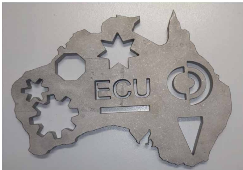
Figure 2. Map of Australia with embedded geometrical shapes cut from an 8 mm thickness AISI 304 L stainless steel plate using abrasive water jet machining (AWJM). (a) Side view. (b) Top view.
