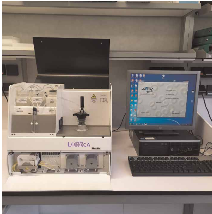
Figure 9. Laser-assisted Optical Rotation Cell Analyzer (LoRRca MaxSis, Mechatronics, Hoorn, The Netherlands) to measure the osmotic gradient ektacytometry (OGE) parameters in hereditary hemolytic anemias.
