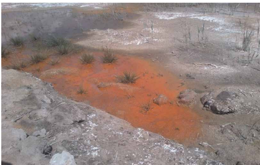
Figure 5. Some AMD and metal precipitation of the floodplain of the right side adjacent to the canal.
