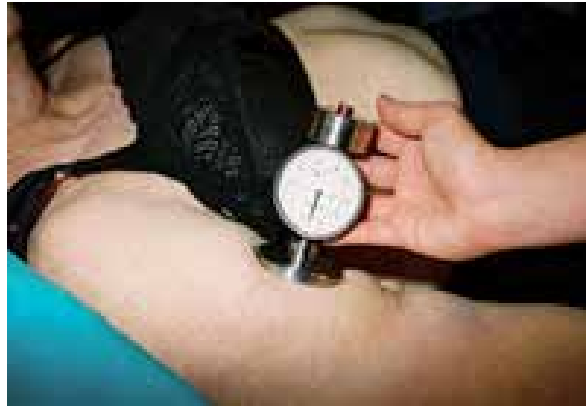
Fig. 3. A tonometer is used to assess the firmness of a tissue by measuring how much force is needed to indent the tissue sample.
