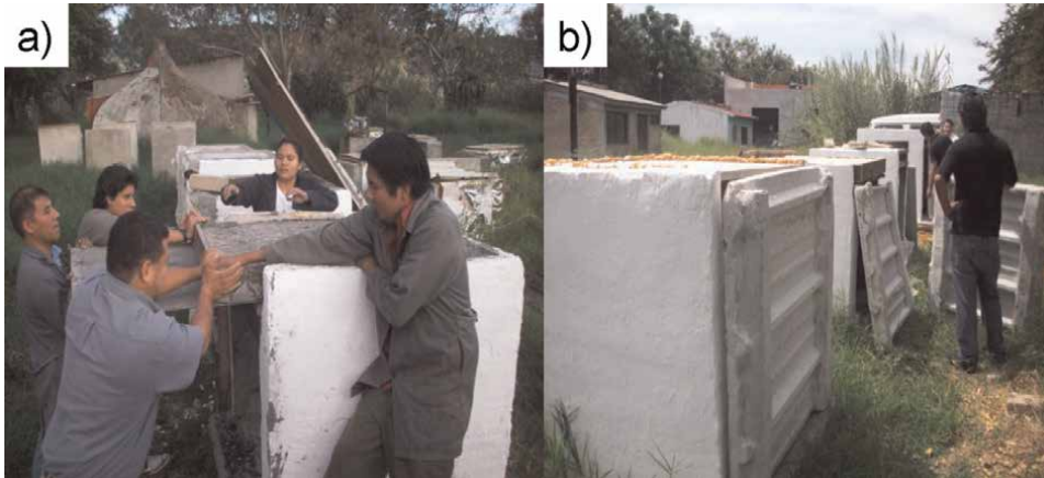
Figure 5. a) Cane bagasse ash panel placement; b) general view of the thermal chambers.
