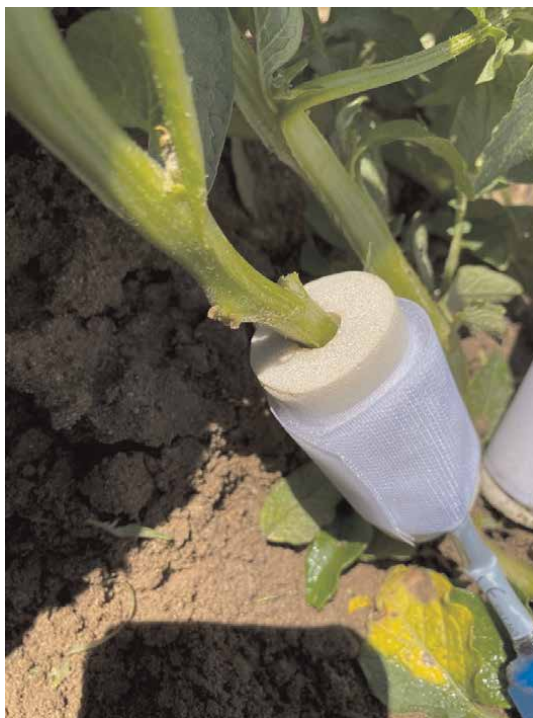
Figure 4. Installed Dynagage flow 32-1 K sap flow system in a potato field (Lakeview, MI, USA).
