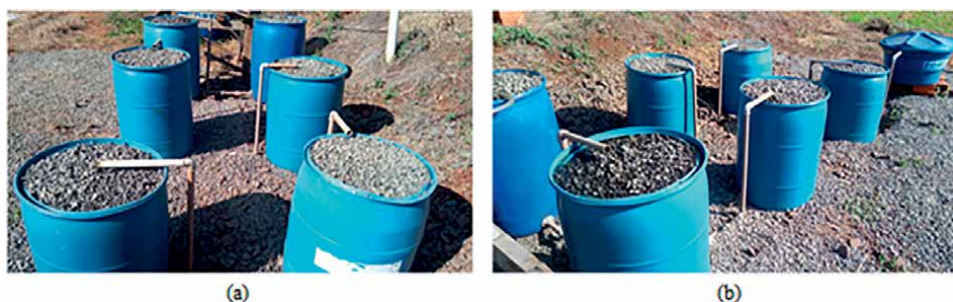
Figure 1. Frontal (a) and lateral (b) view of the WWTP set up at the FCA, UNESP, Botucatu.
