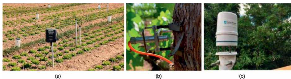
Figure 4. Smart irrigation scheduling approaches. (a) soil sensors for irrigation scheduling, (b) plant sensor for detecting sap flow in plant stems, (c) ATMOS 41 for weather monitoring.
