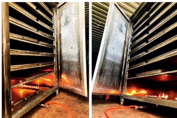
Figure 7. Dry heat from a flame used for the sterilization of growing media.
