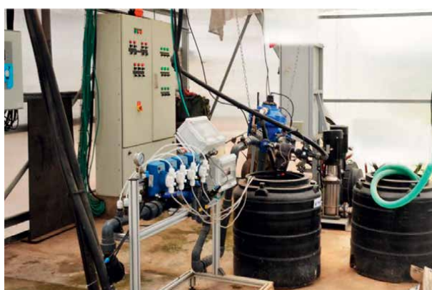
Figure 10. Water and nutrients are applied using a computerized system with sensors and a pre-programmed fertigation regime.
