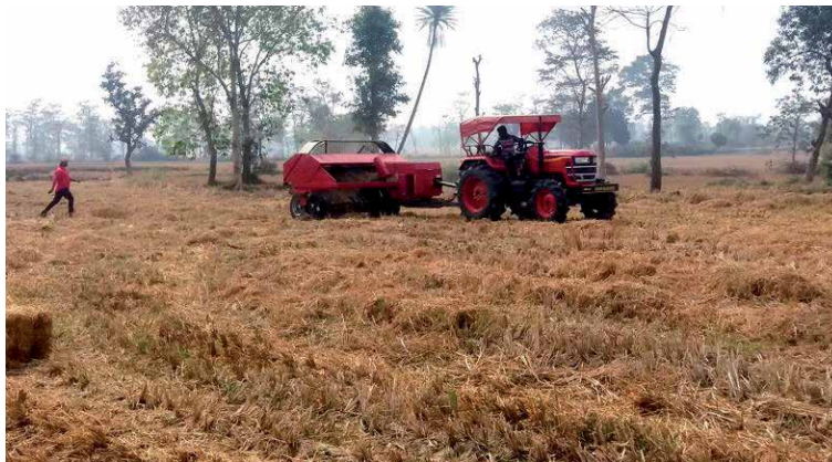
Figure 4. Post harvest operation of square baler in farmer's field in Bargarh district of Odisha, India.
