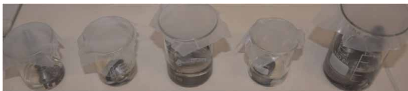
Figure 4. Hydraulic valve samples during test of compatibility with ionic liquids.
