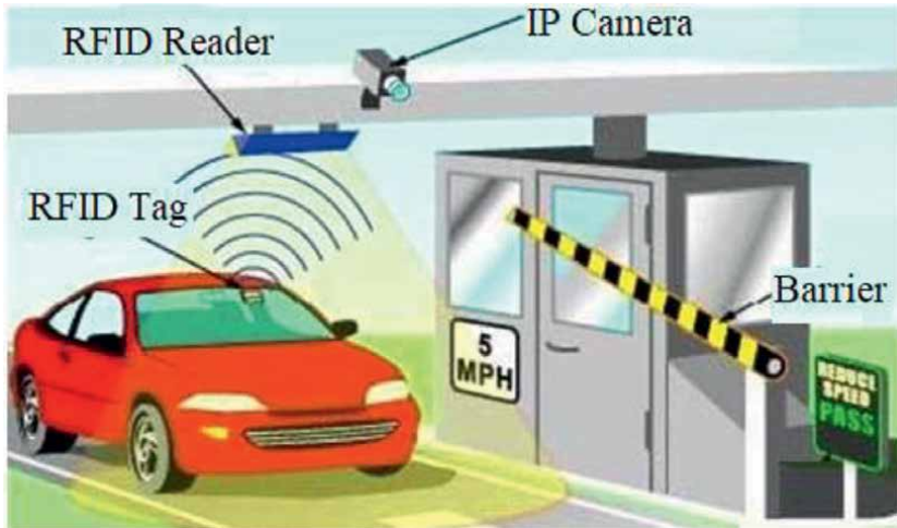
Figure 7. Schematic of a booth in an electronic toll office, which communicates with a passing vehicle.
