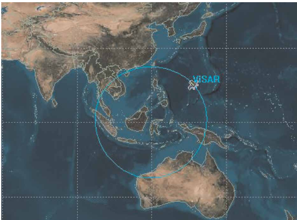
Figure 1. GEOSAR satellite circular trajectory video SAR subsatellite point.
