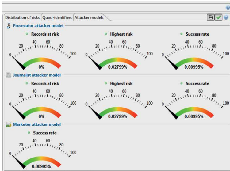
Figure 7. Risk analysis for various types of attacks after applying hybrid privacy preserving data mining (HPPDM) technique for k value = 100.
