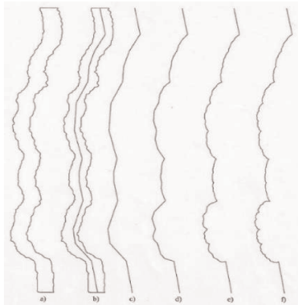
Figure 3. (a) Vectorization of the (b) image with fractal axis and 4 fractal radius increases statuses of the fracture; (c), (d), (e), and (f) (Statuses 0, 1, 2, and 3).
