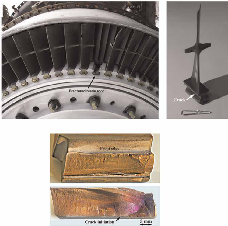
Figure 1. Fracture of a gas compressor turbine blade [16].
