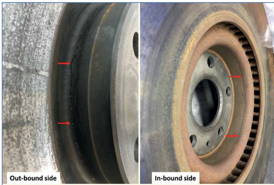
Figure 4. A circumferential crack around the swan neck of the rotor.
