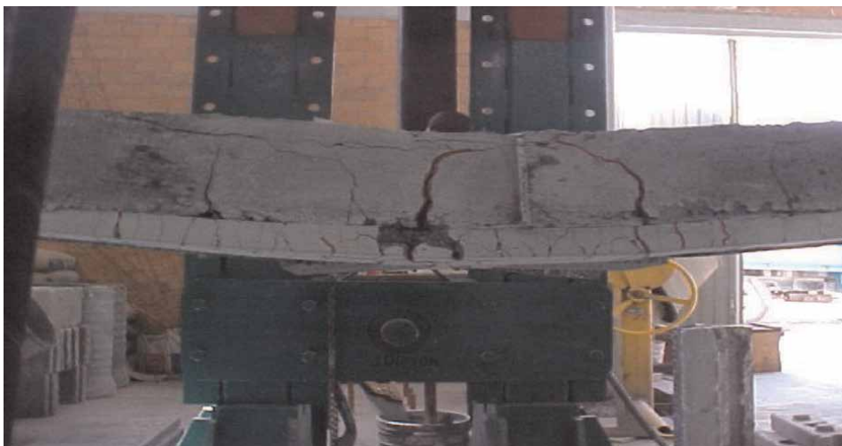
Figure 8. Large deformation and cracking a short time before the collapse.
