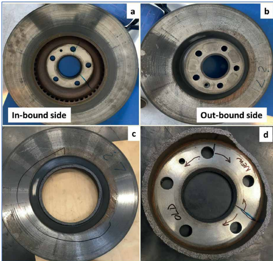
Figure 2. The as-received brake rotor (a) in-board (b) out-board sides of the disc, and (c) and (d) represent the split rotor.
