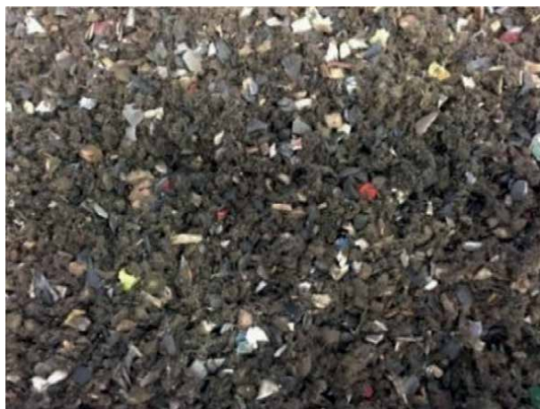
Figure 3. Image of ASR from waste recycling plant. Sourced from ref. [93].
