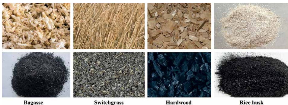
Figure 6. Particles of biochar derived from different feedstocks.
