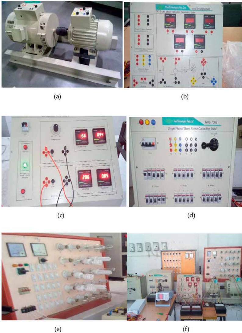
Figure 12. Hardware setup: (a) induction machine coupled with prime-mover, (b) terminals and metering panel, (c) prime-mover motor control panel, (d) excitation capacitor bank panel, (e) load control panel (f) complete experimental set-up.
