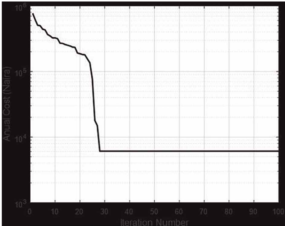
Figure 7. Illustration of annual cost against iteration number for wt/battery configurations [1].
