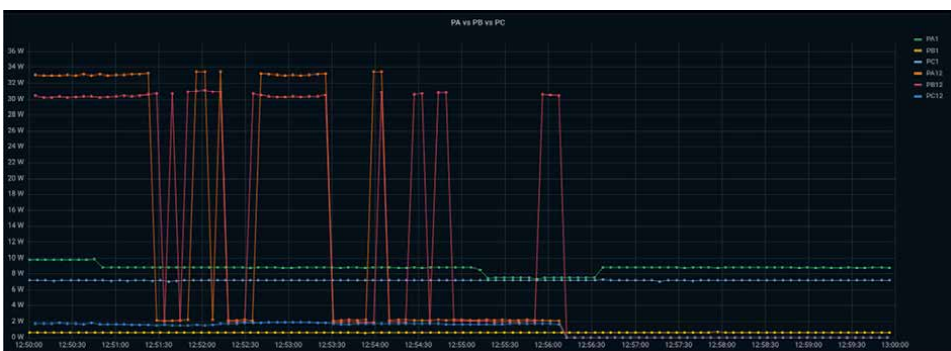
Figure 8. Graphic interface for displaying the active power variations registered by each sensor. Source: prepared by the authors.
