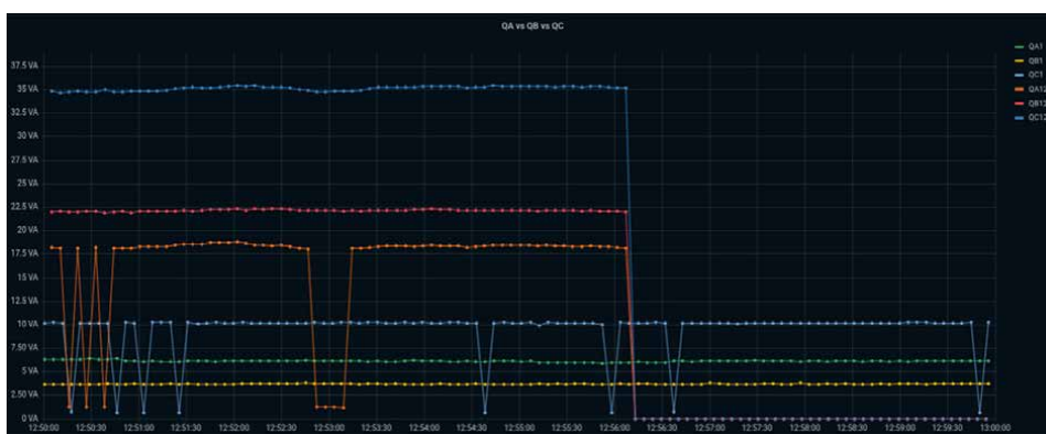
Figure 9. Graphic interface for displaying the active power variations registered by each sensor. Source: prepared by the authors.
