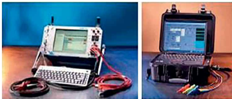
Figure 9. SKF – Baker AWA IV – Offline Test Instrument SKF – Baker (left), The Explorer – Online Test Instrument (right), for electric motor performance monitoring [29].
