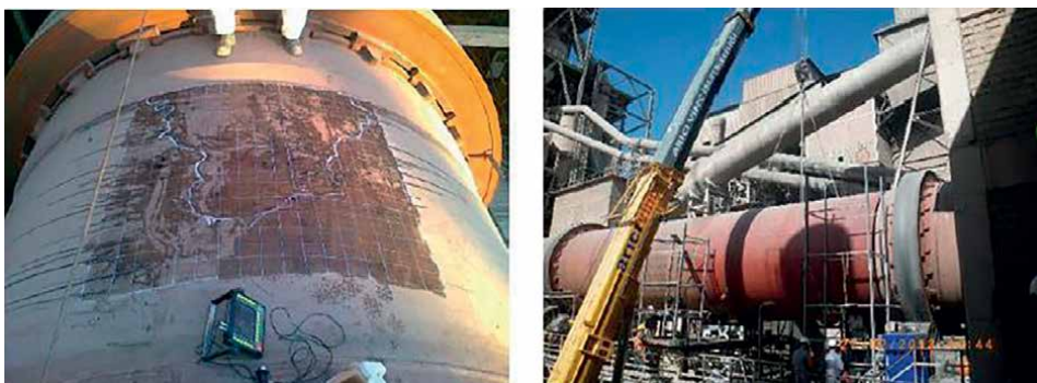
Figure 6. Impairment detection on the cement factory rotating furnace mantle via ultrasonic analysis [19].
