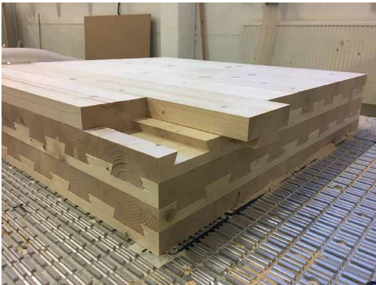
Figure 5. Test specimen of adhesive- and metal fastener-free dovetail wood board element (photo by Hüseyin Emre Ilgin).
